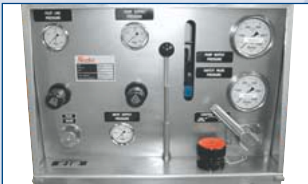
Portable single well control unit
